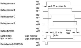
When the muting lamp diagnosis function is enabled, if the muting lamp does not turn on even after 1 second has passed, the muting function will be disabled. When the muting lamp diagnosis function is disabled, the muting sensor will activate 0.05 seconds after the input conditions for the muting sensor A (C) and B (D) are satisfied.
