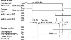
When the muting lamp diagnosis function is activated, if the muting lamp does not turn on even after 1 second has passed, the muting function will be disabled. When the muting lamp diagnosis function is disabled, the muting sensor will activate 3 seconds after the input conditions for the muting sensor A (C) and B (D) are satisfied.
