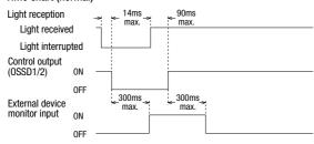
The set time for the device monitoring is 300 ms maximum. Lockout occurs when it exceeds 300 ms. Using the SE9Z-HC controller (optional), setting from 100 to 600 ms (in 10 ms units) is possible.
