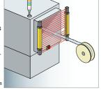
Note: The size of the minimum sensing object changes when the floating blanking function is used.
