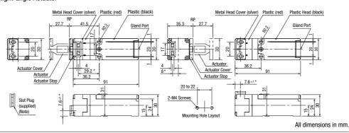
HS5D-□□RN□ (Plastic Head) With HS9Z-A51 Straight Actuator
